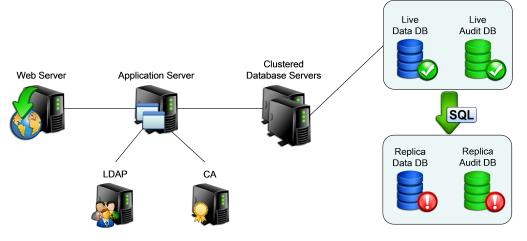
In the example above Microsoft SQL Server Clustering was used to provide failover only, no load balancing was used. In addition the audit database was split out from the main operational database.
