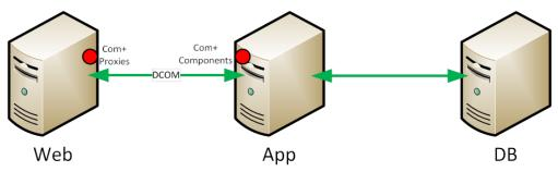
The proxies that run on the web server must be derived from the instance of the components on the individual application server that they are paired with.
