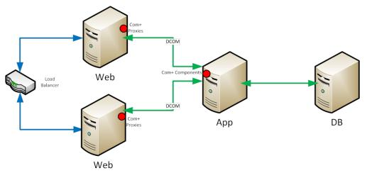
This is OK because each web server (with the COM+ proxies that run it) is still paired with a specific application server. However, this model creates redundancy/failover in the web layer only, meaning that there is still a single point of failure at the application server level.
