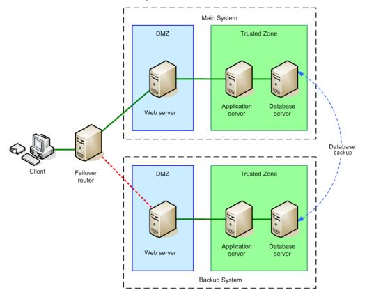
If the database server fails, a manual switch of the failover router would be required. As previously stated, there are many commercially available products for monitoring systems that can do this automatically. Contact customer support for more information.
